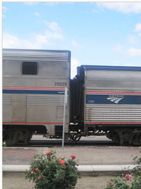
A Superliner transition sleeper with the low er-level connection to a baggage car.
