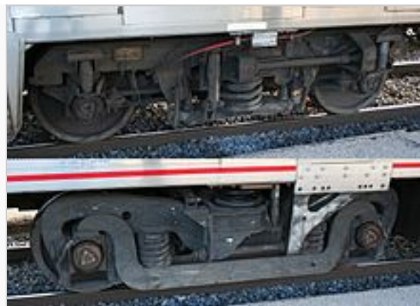
Top: German-designed truck from Superliner I car. Bottom: General Steel Castings truck from Superliner II car.
